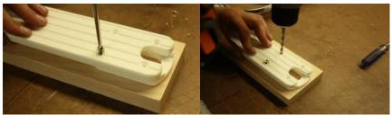
10. Put the drilled fork and tread on the ladder rung. Drop a bolt in one of the holes.
