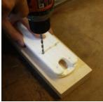
9. Place a bolt through one of the drilled holes to lock the fork and drill all four holes for the fork.
